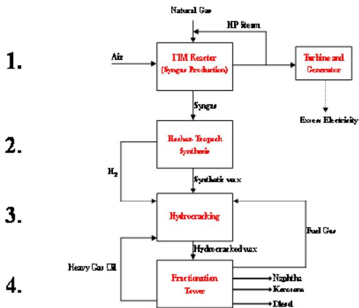
Figure 2. Block Diagram for Overall Process
