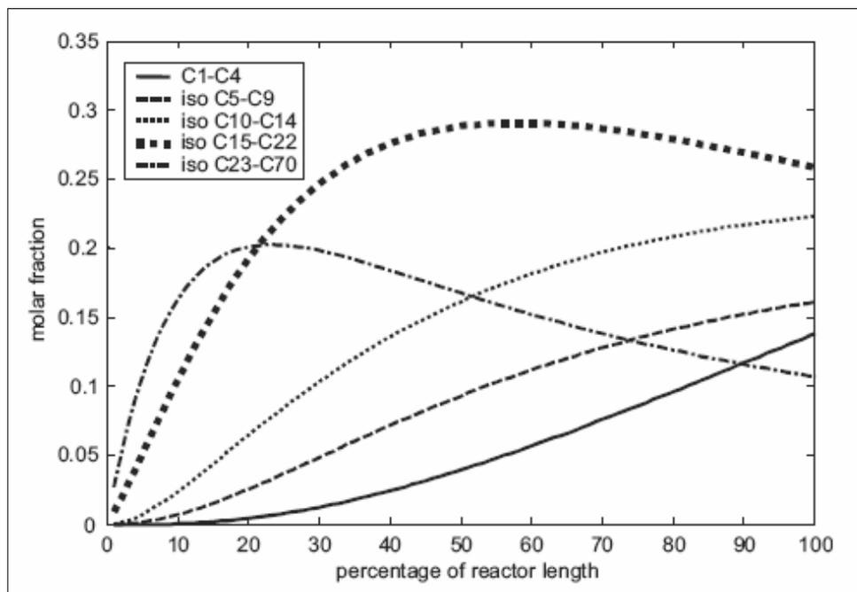
Figure 7. Mole Fractions of Normal Lumps versus Reactor Length (from Pellegrini et al.<sup>1</sup>)
