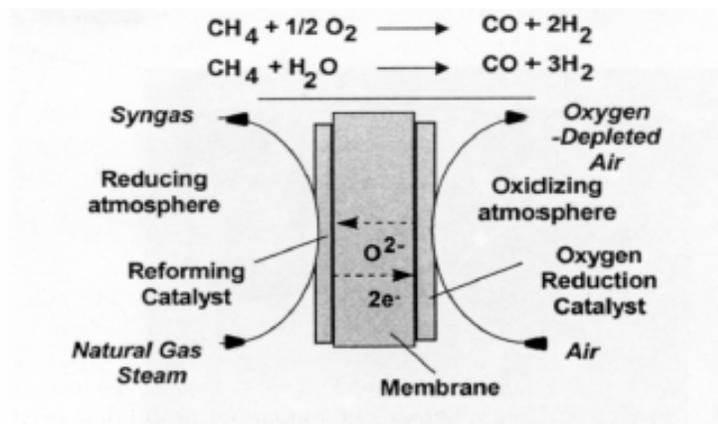
Figure 1. Conceptual Use of an Ion Membrane to Produce Syngas (courtesy of Air Products and Chemicals, Inc).
