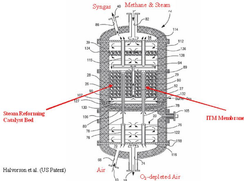
Figure 4. Praxair ITM Reactor Model (2003)
